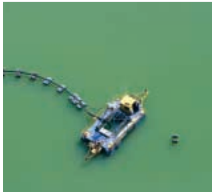
Left: Dredge on Colihues tailings pond.
