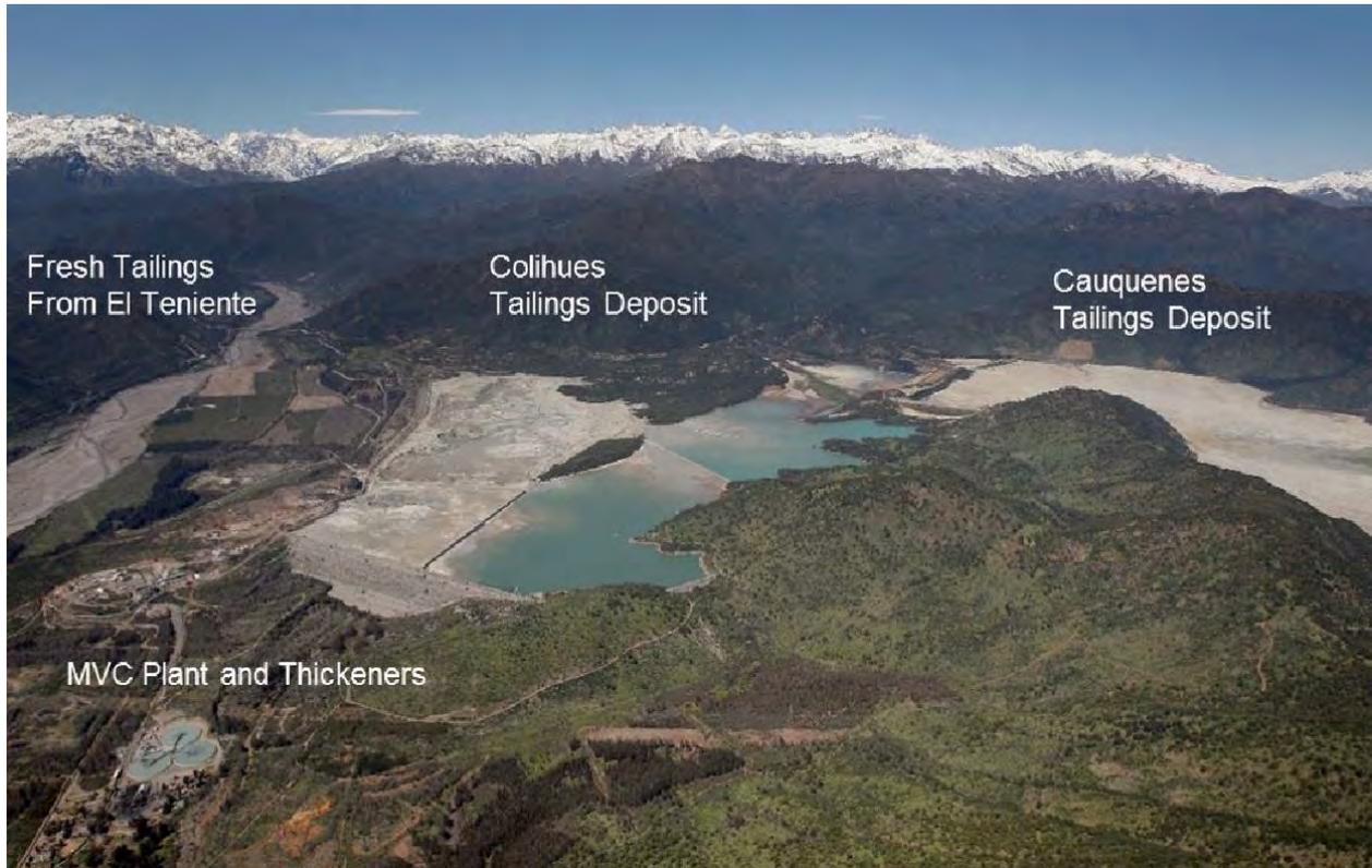
The MVC processing plant has a capacity of 185,000 tonnes per day (tpd) and consists of grinding and flotation to recover copper and molybdenum concentrates. Once the tailings have been reprocessed by MVC, they are returned to the El Teniente tailings launder and transported to the Carén tailings facility located approximately 50 km to the west of the MVC site. Photo 4-2, Photo 4-3, and Photo 4-4 present photographs of the MVC plant layout.
